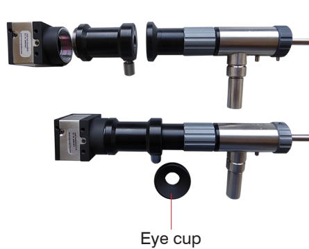
Fig. 10 Assembling the SKF-D endoscope
