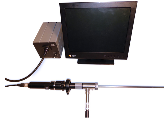
Fig. 17 Final assembly of the endoscope, inclusive analog camera, laptop and light source
