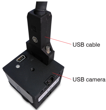
Fig. 14 Connecting the USB camera with the USB cable
