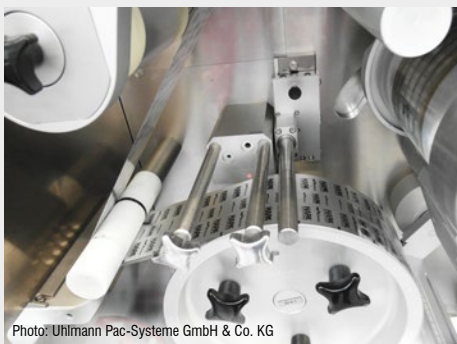
Foreign body detection in blister packs
