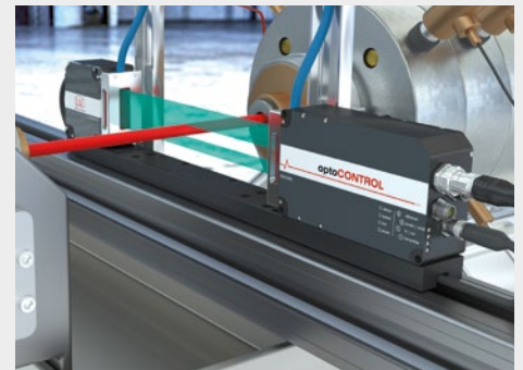
Diameter measurement of extruded products
