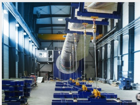
Measuring the deformation of rotor blades for wind turbines
