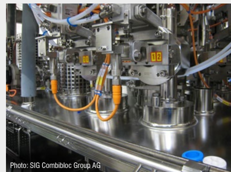
Valve lift measurement in the food industry
