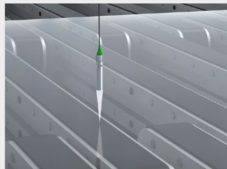
Thickness measurement of flat glass
