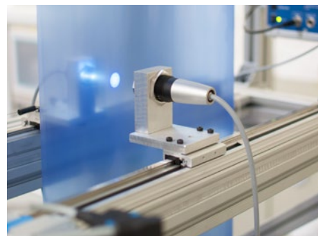
Inline color gradient measurement of transparent film and acrylic glasses
