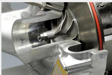
Rotational speed measurement of turbochargers
