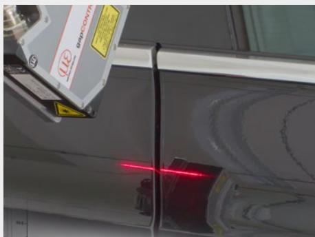
Gap and flushness measurement on bodywork parts
